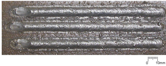
Fig. 11. Welds made using E7018 electrodes demonstrating the flexibility and repeatability of the process.
