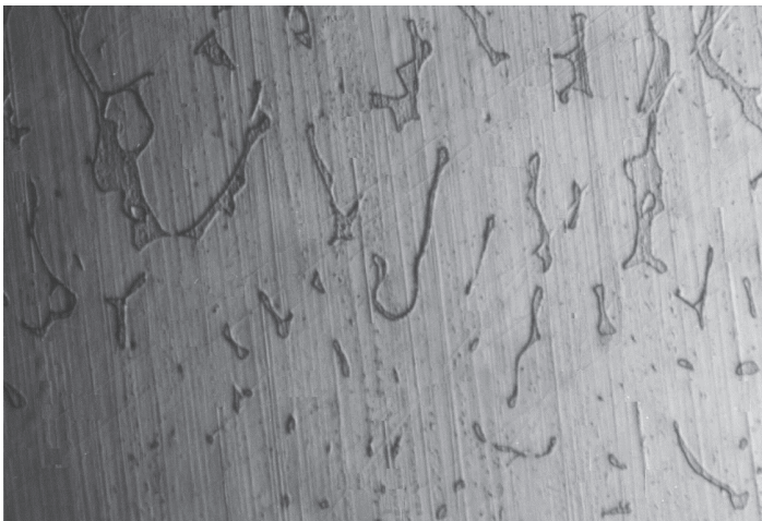
Fig. 14. Micrograph showing the two-phase austenite + vermicular delta ferrite mixture in the weld metal of 309L stainless steel. Etching: (HCl/HNO 3 ) reagent. Magnification: 1600x.
