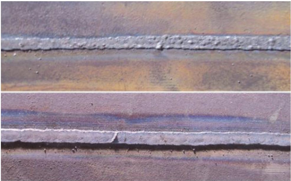
Fig. 8. Back view of welds from inside the pipe; for Ex.1 (up) and for Ex. 2 (down), Ex. 2 has more penetration than Ex. 1 related to the more WHI
